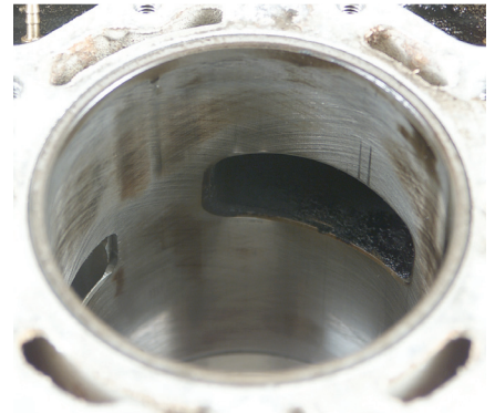
This photo shows one of the cylinders from the hp Injector-lubricated engine. Note that the original cross-hatch pattern is still visible. The scratch marks above the exhaust port are the result of a mechanical phenomenon; they appear in the exact same spot on the XD100-lubricated cylinders.
